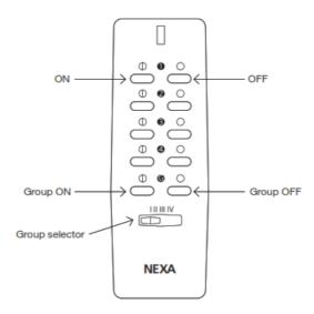
The remote control has 16 channels divided into 4 groups. Use the Group ON/Group OFF button to switch all the channels in a group on or off.
