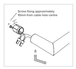
Typical wiring for timber framed walls is Ihe distance from the transformer to the furthest 12V connection should be no more than 2000mm. Make sure that the 12V cabling doesn't cross the 230V mains cable. Insulation should be removed from the vicinity of the transformer toa radius of 150mm. The single bar heated towel rail is designed as dual wire option (left or right hand)- nect one Side only.
