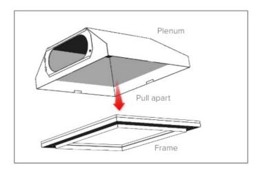
If the diffuser is located inside the ceiling cavity, access it through ceiling hole, and detach frame. Alternatively, feed the frame through the ceiling hole as shown below
