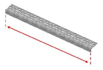
Cut length of edge bead to match frame opening. For best result, gaps should be minimal Install 4x edge beads to ceiling opening. Fasten and set into ceiling as per standard plastering practices
