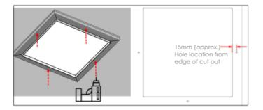
Use impact driver to secure with 4 x screws (8g x 20 countersunk)
