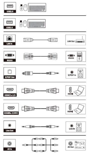
• **Note** Please do not connect a 2.4G wireless mouse and USB 3.0 devices simultaneously, on the left back side of the display, to avoid interference.
