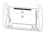
2. Remove the left and right screws 1 (4 pcs) and install the lifting handle 2 (4 pcs):
