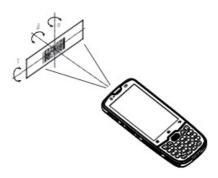
Adjust the scan angle and the distance between the PDA and the target barcode to make them fall into the following ranges:
