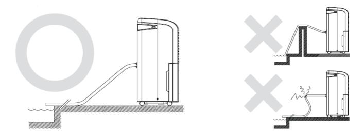
**Option 2**Automatic pump-out operations Installation:
