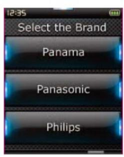
2. Once the brand has been selected, you can then search through the available codes for that brand by trying keys on the remote. If the keys respond correctly, you can accept the current code by pressing "Works", or test the next code by pressing "Next". When the device has been set up, you will have the option to set up another device.
