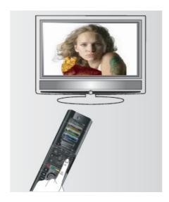
If the device responds as expected, press the function key labeled "Works". If the device does not respond, either try a different key or press the function key labeled "Next" to test the next device code.
