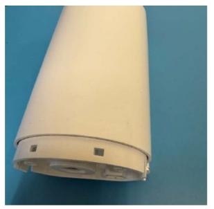
3. The connection of the two modules is completed when the radio and sensor module 'snaps' into place within the upper enclosure. The pictures below show the approximate depth required for the 'snap.'
