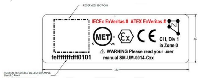
Representative Label for the Lid, Radio and Sensor Module (26-000023-DWG).
