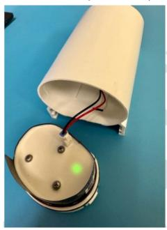
2. Align the radio and sensor module and the power module and begin sliding the two together. The radio and sensor module will fit inside of the power module.
