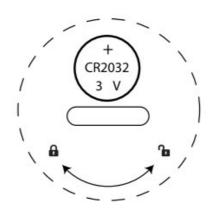
Use a tool to open the battery cover and insert the battery according to the "+/-" symbol marked in the battery compartment (CR2032 or CR2025 is common.) If you do not plan to use the remote control for a long time, please remove the battery
