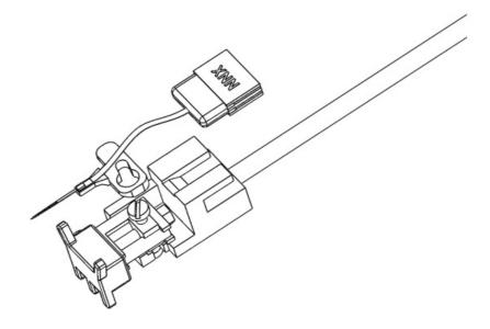
**Step 5**Push the front screw through the larger probe mount screwhead opening.
