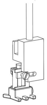
**Step 3** Tighten the screw to lock the nDrive onto the IST-nDrive.
