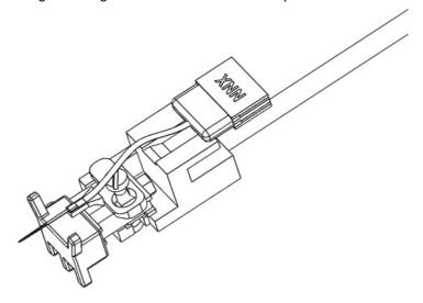
**Step 7** Place the probe connector into the connector bracket.
