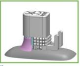
11. Gather any exposed flex cable and place the connector into the remaining hooks on the drive cap. Attach any exposed reference wires now.
