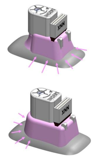
13. After the cement is fully cured, the device is ready for use. Adjust the electrode depth with the provided 1.8 mm slot screwdriver. The adjustment screw pitch is 250 µm per turn.
