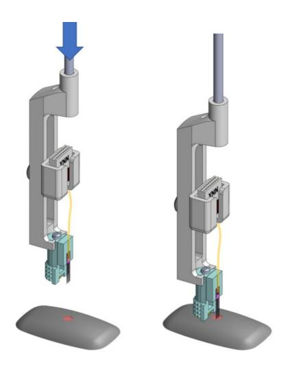
4. Prepare a small amount of dental cement. The first application of cement is only meant to hold the drive during head cap installation and should be minimal. Cement must not be applied outside the indicated area.
