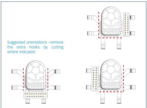
10. Lower the protective cap (shown with side hooks removed) into place on top of the drive, aligned as shown. The cap must be fully seated before continuing.
