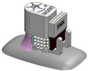
12. Prepare a batch of dental cement. Apply cement liberally to the perimeter of the device, ensuring to bury any exposed flex cable or reference wires/screws for protection. Any remaining knurl should be covered with dental cement.
