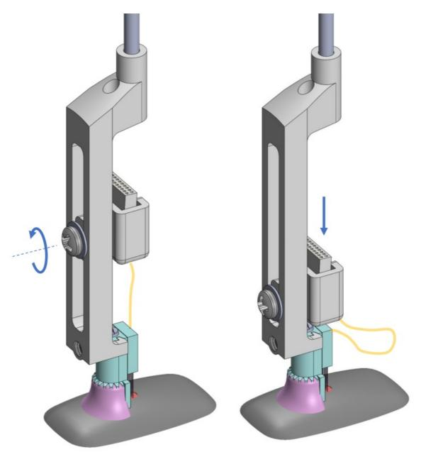
7. Remove the package from its holder. A helping hand/third hand may be used to keep the package in a fixed position (to avoid unnecessary stress on the flex cable).
