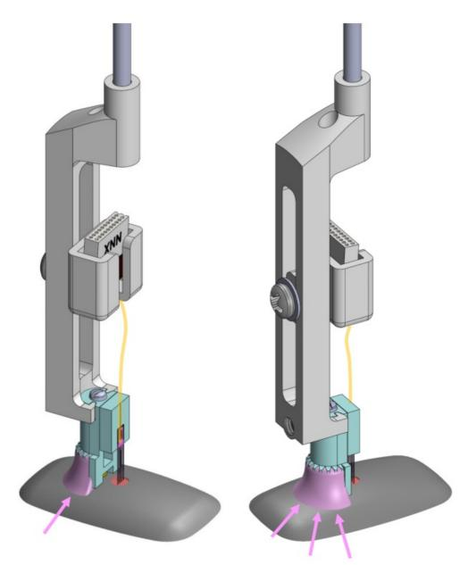
6. Loosen the package holder screw with the provided #0 Phillips screwdriver. Slide the package holder downward (towards the skull) in its track to create slack in the flex cable.
