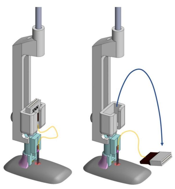
8. Using the provided 0.9 mm Hex screwdriver, loosen the set screw on the rear of the drive 2-3 complete revolutions to release the drive from its insertion holder. Retract the holder away from the drive using your stereotaxic frame.
