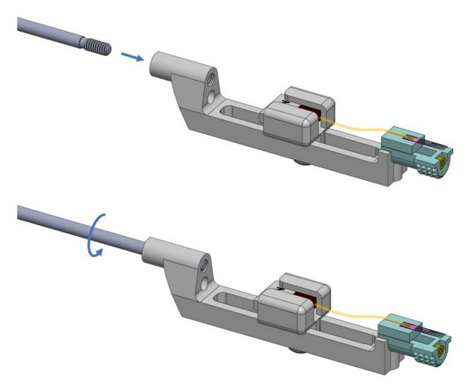
3. Attach the 2 mm rod to your stereotaxic inserter over your prepared craniotomy. Lower the device along the insertion path until it meets the skull. Depending on your electrode offset, the shanks may be partially implanted during this process.
