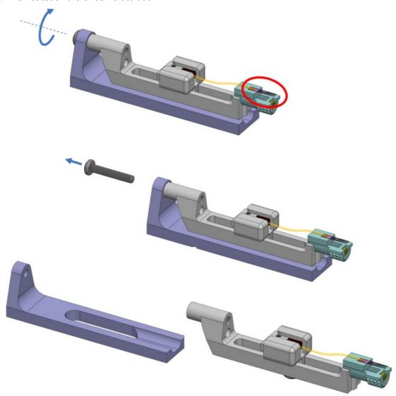
2. Attach an M2 threaded stereotaxic rod. This rod is coaxial with the electrode and will be used to manipulate and implant the device during this procedure.
