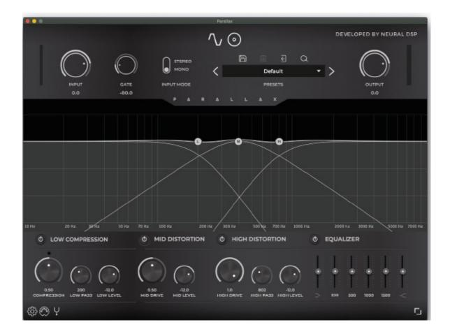
Parallax is a multi-band distortion for bass. This plugin is meant to bring the user a ready tool, which is based on a studio technique used by audio engineers and producers to craft their bass tone. Bass, mids, and high frequencies are processed separately with distortion and compression to be mixed back together.
