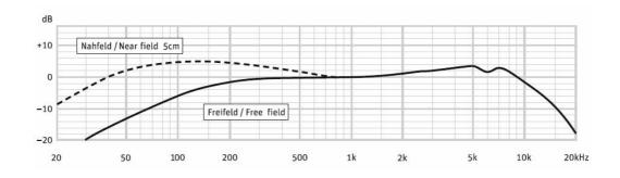
measured in free-field conditions (IEC 60268-4) into 10 kohm rated load impedance
