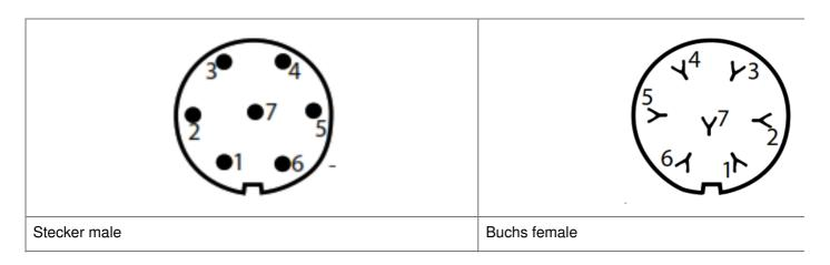
The included seven-core KC 5 cable connects themicrophone to the pattern control unit NM V.
