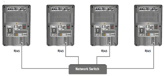
This device supports Sennheiser Sound Control (SSC) based on TCP and IPv6. The static IPv6 address of the device can be determined with mDNS. For more information about SSC, see the Sennheiser website.
