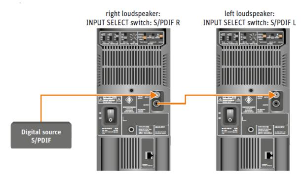
The settings of the first loudspeaker in the signal chain are not looped through to the second loudspeaker. Each loudspeaker must be configured separately.
