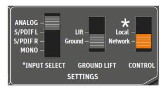
If the CONTROL switch is set to Network but there is no network connection and the MA 1 – Automatic Monitor Alignment software is not active, the most recent network configuration is used.
