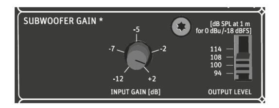
To do so, use the potentiometer SUBWOOFER GAIN | INPUT GAIN 12 and the switch SUBWOOFER GAIN |
