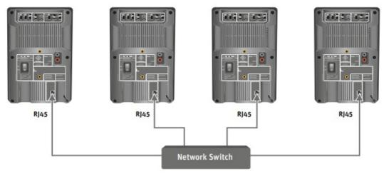
**info:** This device supports Sennheiser Sound Control (SSC) based on TCP and IPv6. The static IPv6 address of the device can be determined with mDNS. For more information about SSC, see the Sennheiser website.
