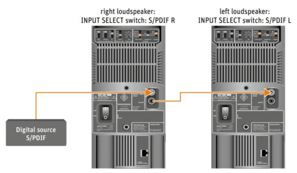
• **info:** The settings of the first loudspeaker in the signal chain are not looped through to the second loudspeaker. Each loudspeaker must be configured separately.
