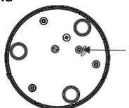
Small bottom screw at the base of device pointed by an arrow.
