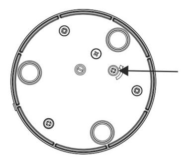
The small bottom screw at the base of the device is pointed by an arrow.
