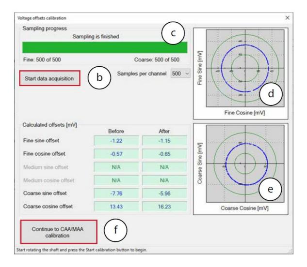
• When offset calibration is completed, click on <Continue to CAA/MAA Calibration> button (f).
