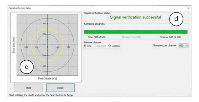
Note how ever, that mounting the encoder towards the extreme mechanical tolerances might cause the amplitude circle to be offset from the exact middle of the nominal position.
