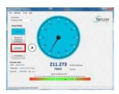
For optimal performance of the Electric Encoders, the inevitable DC offset of the sine and cosine signals must be compensated over the operational sector.
