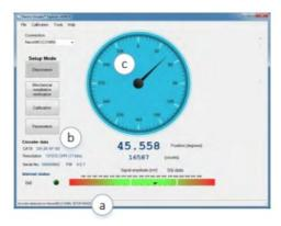
Perform mounting verification & rotation direction selection before calibration to ensure optimal performance. Observing the installation at the [Tools – Signal Analizer] window is also recommended.
