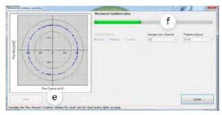
At the end of a successful verification, the SW will show "Correct Mechanical Installation."
