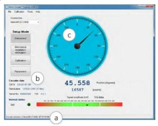
Perform mounting verification & rotation direction selection before calibration to ensure optimal performance. It is also recommended to observe the installetion at the [Tools – Signal Analizer] window.
