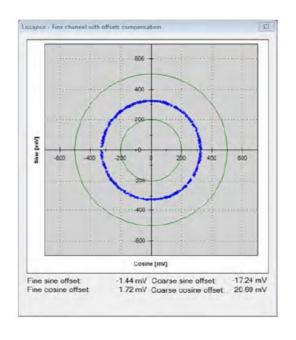
Mechanical compensate by using 50 um shims below the rotor (available as DS-130-R-00 kit). Verify proper rotor mounting with the Encoder Explorer tools "Signal analyzer" or "Mechanical installation verification."
