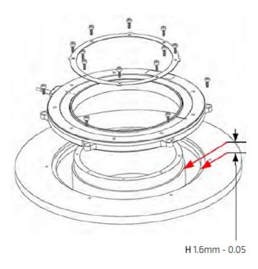
The rotor is floating, therefore, for proper relative axial mounting distance "H" between the shaft shoulder (b) and stator mounting recess (a) should be 1.5 mm nominal. For ease of mechanical mounting compensation by rotor shims, the recommended distance is 1.6-0.05 mm. The optimal recommended amplitude values are middle of the range according to those shown in the Encoder Explorer software and vary according to the encoder type.
