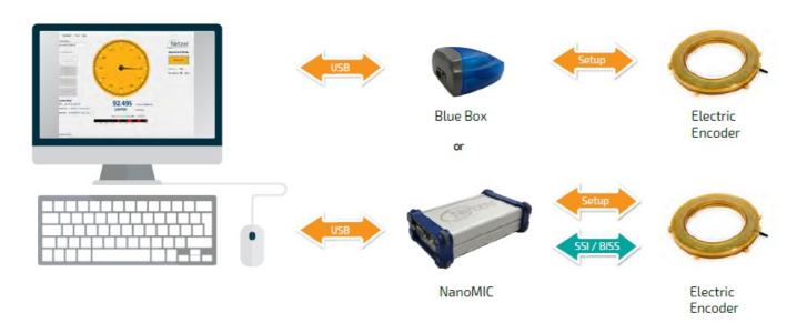
Connect Netzer encoder to the converter, connect the converter to the computer and run the Electric Encoder Explorer Software Tool.
