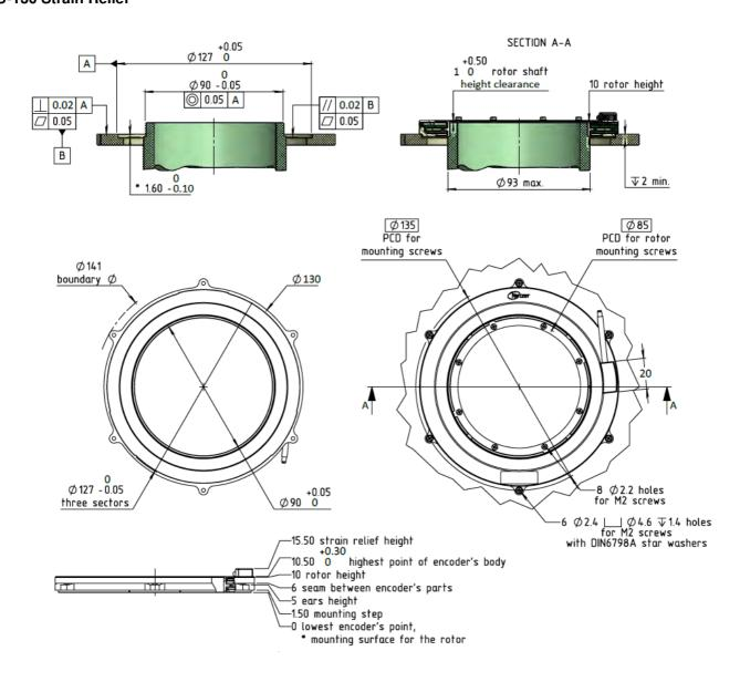
**WARNING:** Do not use Loctite or other glues containing Cyanoacrylate. We recommend using 3M glue – Scotch-WeldTM Epoxy Adhesive EC-2216 B/A.
