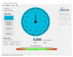
The zero position can be defined anywhere in the working sector. Rotate the shaft to the desired zero mechanical position. Go into the "Calibration" button at the top menu bar, press "Set UZP". Select "Set Current Position" as zero by using the relevant option, and click [Finish].
