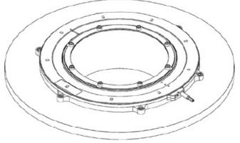
The encoder rotor (2) attaches to the host shaft by pressing it against a dedicated shoulder (b). A screw and washer or circular spring and washer at the end of the shoulder maintain pressure. The encoder stator (1) is centered by circumferential step (a) and attached to the host stator (c) using six M2 screws, recommended torque of 0.3Nm.
