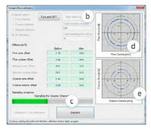
• Start the data acquisition while rotating the shaft. The progress bar (c) indicates the collection progress. Rotate the axis consistently during data collection-covering the working sector of the application end to end-by default the procedure collects 500 points over 75 seconds. Rotation speed is not a parameter during data collection. Data collection indication shows for the fine/coarse channels, a clear "thin" circle appears in the center (d) (e) with some offset.
