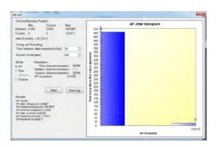
Perform a jitter test to evaluate the quality of the installation; the jitter test presents the reading statistics of absolute position readings (counts) over time. Common jitter should be up +/- 3 counts; higher jitter may indicate system noise.
