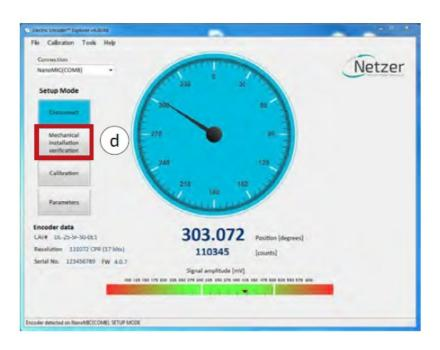
The Mechanical Installation Verification provides a procedure that will ensure proper mechanical mounting by collecting raw data of the fine and coarse channels during rotation. (d) Select [Mechanical Mounting Verification] on the main screen.
