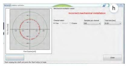
• If the SW indicates "Incorrect Mechanical Installation," correct the mechanical position of the rotor, as presented in paragraph 3.3 – "Rotor Relative Position."
