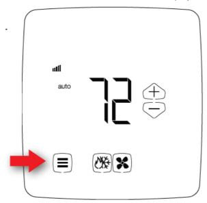
2. Next, press the hidden button, located to the left of the Checkmark button. This will retrieve the device name. The device name will be displayed in the Dot Matrix of the faceplate.
