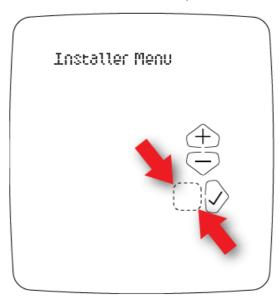
3. Use the Checkmark button and the Return button to switch between the Thermostat Name, IP Address, and MAC Address. WRITE DOWN THE IP ADDRESS. To exit the menu, tap the Cancel button at the bottom right of the display.
