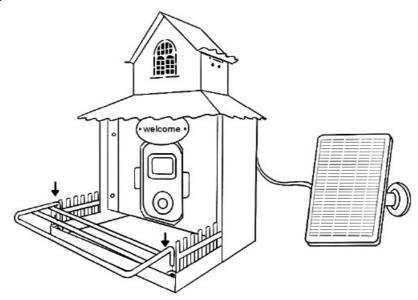
10. Install solar panels in a place with sufficient sunlight
