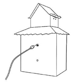
4. Open the door card and let the solar panel wire pass-through
