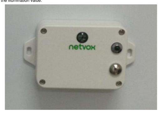
**Note:** Please do not disassemble the device unless it is required to replace the batteries. Do not touch the waterpro of gasket, LED indicator light, function k eys when replacing the batteries. Please use suitable screwdriver to tighten the screws (if using an elect ric screwdriver, it is recommended to set the torque as 4kgf) to ensure the device is impermeable.
