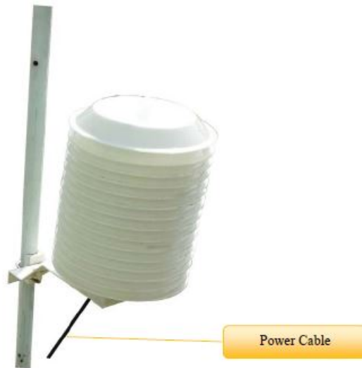
Fig. 3. RA0723Y shield is equipped with PM2.5, temperature and humidity sensor and noise sensor
