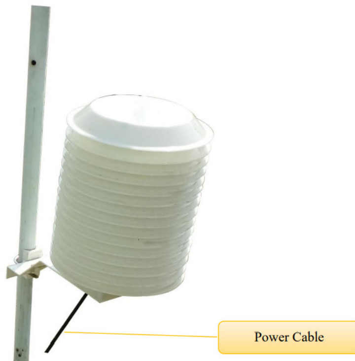
Fig. 3. RA0723Y shield is equipped with PM2.5, temperature and humidity sensor and noise sensor (subject to the actual object).
