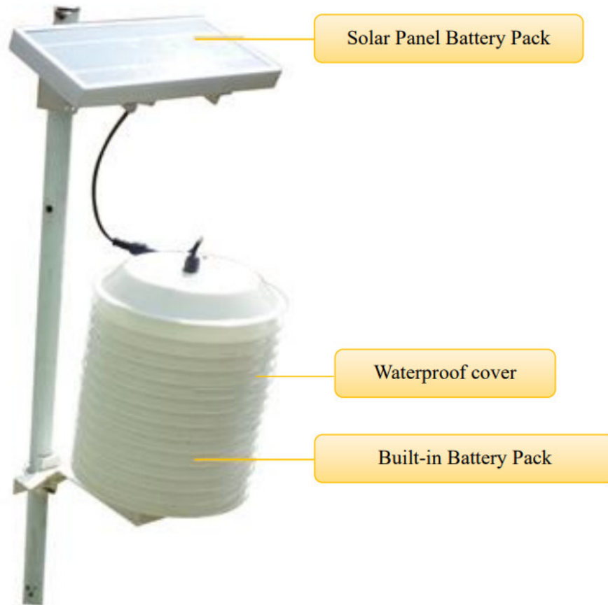
Fig. 2. R72623 shield is equipped with PM2.5, temperature and humidity sensor and noise sensor (subject to the actual object), external solar power supply.
