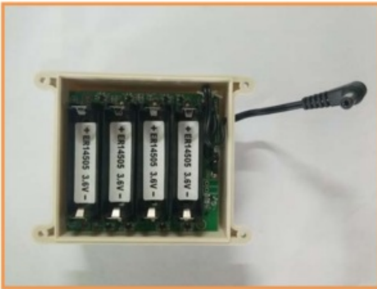
Figure 2. The reverse side of the battery PCB
