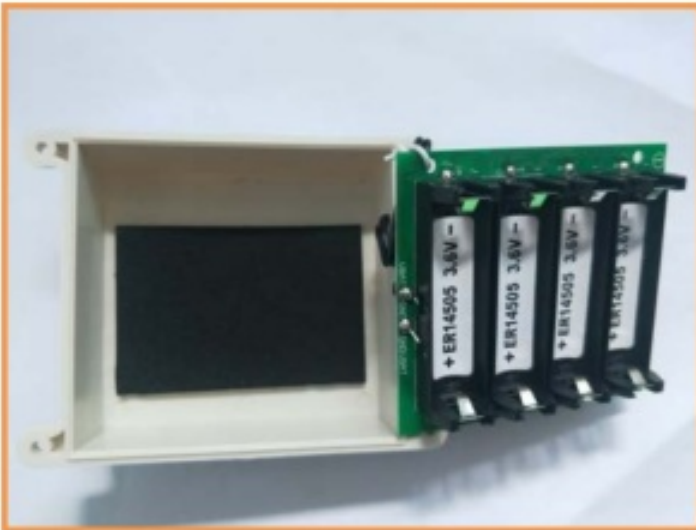
Figure 2. The reverse side of the battery PCB
