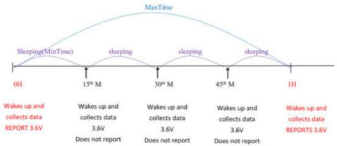
**Example#3** based on MinTime = 15 Minutes, MaxTime= 1 Hour, Reportable Change i.e. BatteryVoltageChange= 0.1V.
