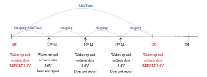
**Example#3** based on MinTime = 15 Minutes, MaxTime= 1 Hour, Reportable Change i.e. BatteryVoltageChange= 0.1V.
