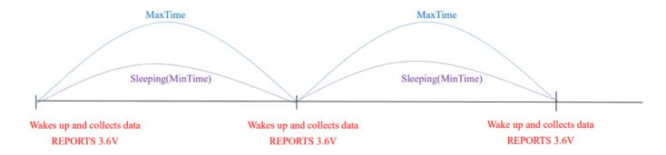
Example#2 based on MinTime = 15 Minutes, MaxTime= 1 Hour, Reportable Change i.e. BatteryVoltageChange= 0.1V.
