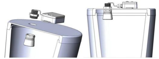
5. If the top of the water tank cannot be opened, the hole made on the top of the water tank is recommended to be 45mm diameter. It is recommended to add a gasket (size: 32.4\*57.4\*3mm) between the hole and the sensor.
