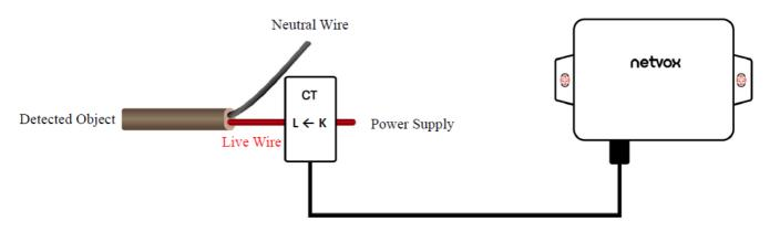
CT Wiring Schematic Diagram (Current direction K→L)
