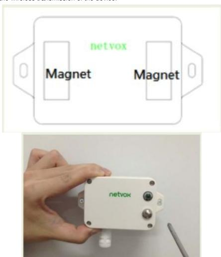
2. Tear off 3M release paper of Hall sensor and the magnet then attach to the door or window in parallel.
