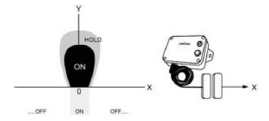
If the magnet moves along the Y axis relative to the sensor, it will cause repeated reports due to the magnetic field.
