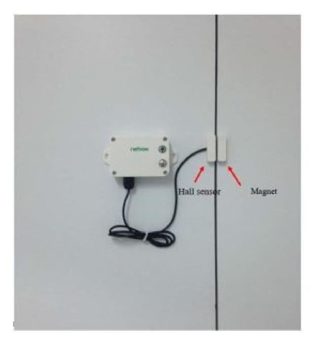
When installing the device, the magnet must move along the X axis relative to the sensor.
