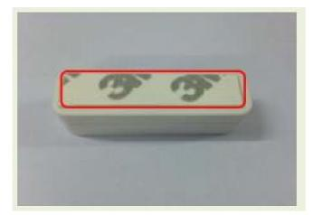
3. When the door or window is opened, the Hall sensor is separated from the magnet, and the Hall sensor sends status "1".
