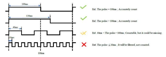
Pulse filtering time must be multiple of 5ms (can be set)
