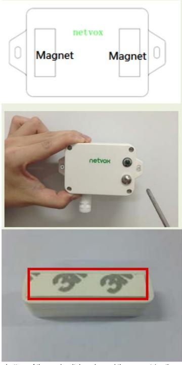
2. Tear off the 3M glue at the bottom of the reed switch probe and the magnet (as the red frame in the figure above). Then, stick the reed switch probe to the door and is parallel to the magnet (as the figure on the right).
