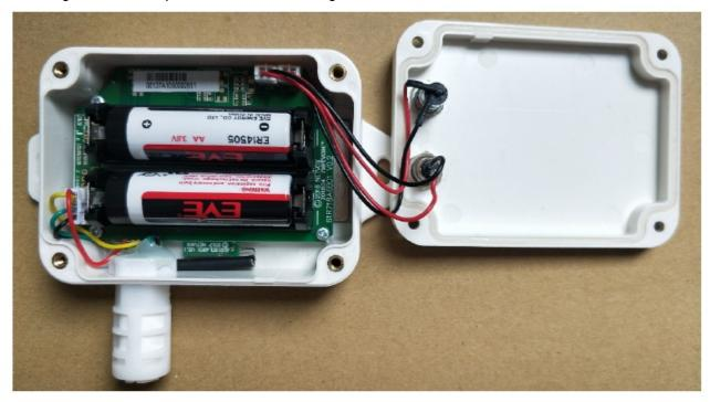
**Note:** Please do not disassemble the device unless it is required to replace the batteries. Do not touch the waterproof gasket, LED indicator light, function keys when replacing the batteries. Please use suitable screwdriver to tighten the screws (if using an electric screwdriver, it is recommended to set the torque as 4kgf) to ensure the device is impermeable.
