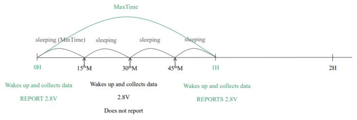
Example#3 based on MinTime = 15 Minutes, MaxTime= 1 Hour, Reportable Change i.e. BatteryVoltageChange= 0.1V.
