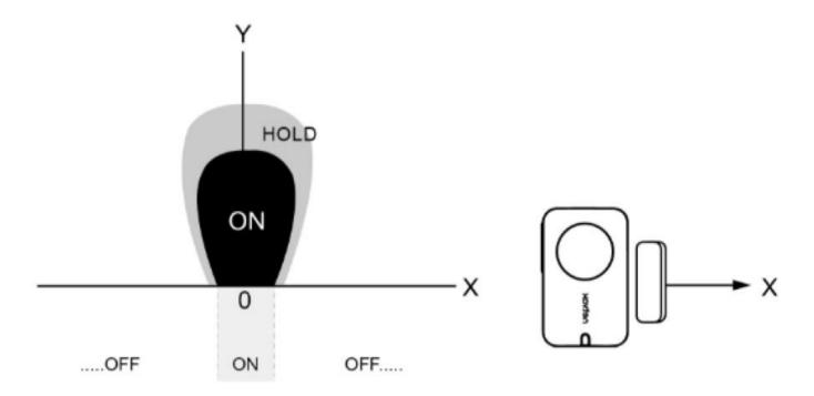
If the magnet moves along the Y axis relative to the sensor, it will cause repeated reports due to the magnetic field.
