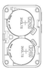
Note: To install the battery, use a screwdriver or similar tool to assist in opening the battery cover.
