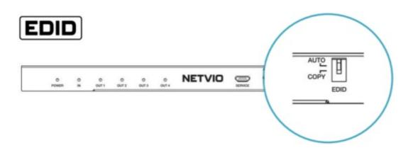
When copying EDID, connect your display device to Output-1. Recycle power every time settings are adjusted.
