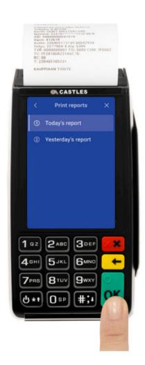
Press the power/menu key in the left corner of the terminal for displaying the menu on the terminal screen. Choose [4], Reports.
