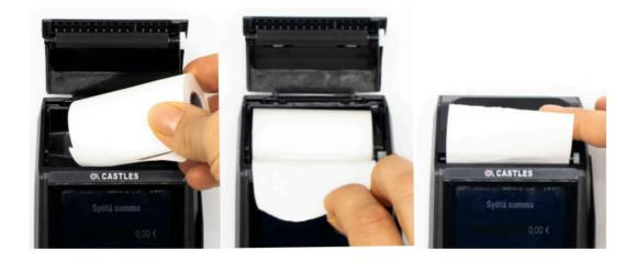
Install the receipt paper roll (57×40mm) in the compartment by opening the lid of the receipt roll cover by lifting the cover up. Discard any packing material from the paper roll. Place the roll in the compartment as shown in the figure.
