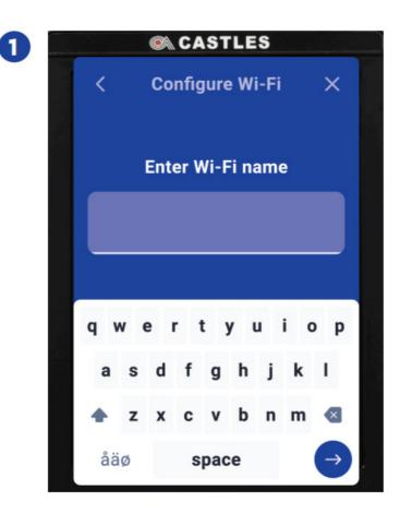
Enter the Wi-Fi name (SSID) using the virtual onscreen keyboard. Please, ensure that the uppercase and lowercase letters are entered correctly. Accept the value using the green [OK] key. The terminal will then prompt for the Wi-Fi passphrase (PSK):
