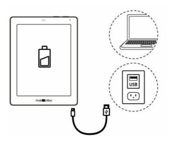
• **Charging:** connect the supplied Type-C charging cable to the MobiScribe. The MobiScribe can be charged via a wall outlet (USA power adapter is not included), or via a USB port.
