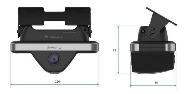
Driveri™isan AlpoweredvisionbasedIoTsystem,soldasanaftermarketproducttofleets. The device is installed in trucks/cars behind the rear-view mirror, and the power is supplied from the car battery through a custom power cable.
