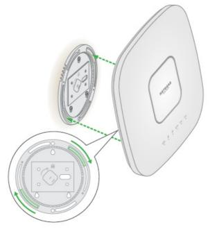
8. Twist the AP clockwise to lock it onto the mounting plate.
