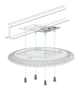
7. Hold the AP upside down and attach it to the mounting plate.
