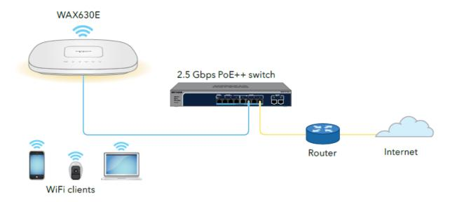
If connected to 2.5 Gbps equipment, the WAX630E LAN 1/PoE++ port supports Ethernet speeds up to 2.5 Gbps
