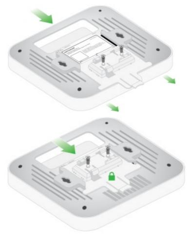
**Note:** To unlock the access point, push the locking tab toward the ceiling and slide the access point out of the bracket.
