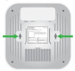
1. Mark the wall where you want to insert the provided anchors and screws, which must be 3.87 in. (98.5 mm) apart, and insert the anchors and screws.
