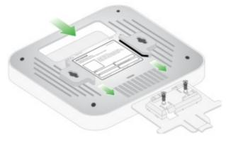
3. Slide the access point into the bracket until it locks in place. The locking tab must be at the front of the access point.
