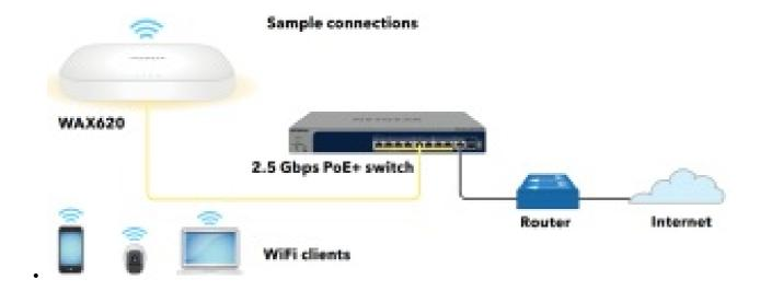
The access point receives an IP address from a DHCP server (or a router that functions as a DHCP server) in your network. If your network does not include a DHCP server, the access point uses its default IP address 192.168.0.100.
