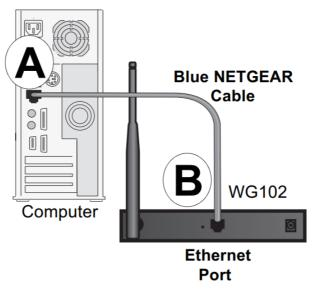
• c. Connect an Ethernet cable from the WG102 to the PC (point A in the illustration).
