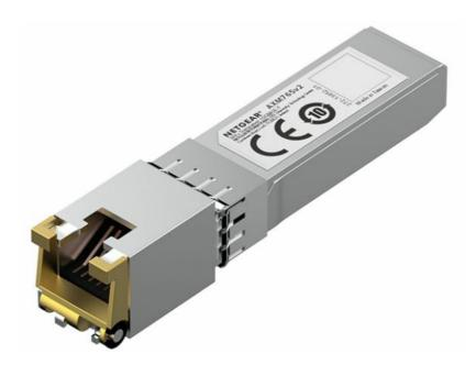
The AXM765 SFP+ module is a low-power, high-performance, multi-gigabit 10G/1000BASE-T transceiver. The AXM765 delivers 10 Gb network connectivity with cabling up to 98.5 feet (30 meters) and delivers 1G network connectivity speed through 328 feet (100 meters) of Category 5e (Cat 5e) or Cat 6 Ethernet cable.
